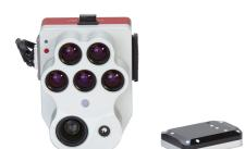
**AgEagle RedEdge Altum-PT:** The 3-in-1 sensor offers a high-resolution, five-band spectral imaging solution tailored for intricate remote sensing in agriculture and archaeology, and works seamlessly with the M300 drone.
